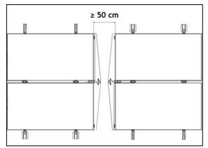
IMPORTANT! Make sure there is enough space planned in between the arrays. This space is required to mount the side deflectors.
