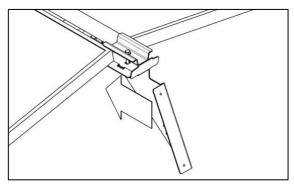
1. Slide the bracket with the clamp in between the modules at the top.
