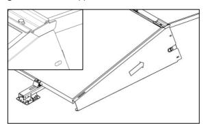
8. Slide the deflector up against the notch on the bracket. Check if the slot on the low side aligns with the clamp. Adjust the position of the clamp when necessary.
