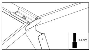
2. Tighten the bolt on top.
