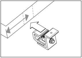
3. Hook the clamp on the module frame on the low side. Place the clamp roughly 5 cm from the corner of the module.
