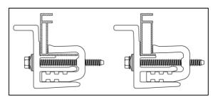
Note: The clamp can be used for multiple types of module frames as shown below.
