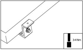
4. Tighten the pre-assembled screw in the clamp.
