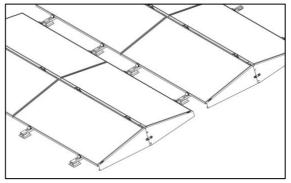
11. Install the deflectors on all open sides of the interconnected field.
