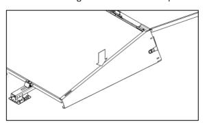
7. Hook one of the deflectors on the clamp and bracket. Place the cables in the cable grommet, when applicable.
