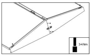
10. Mount the 4 short screws: two in the bracket and in each clamp one.
