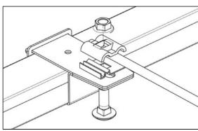
3. Insert the M10x25 carriage bolt from below into the slot hole. Assemble the ground clamp together with the lightning conductor.
