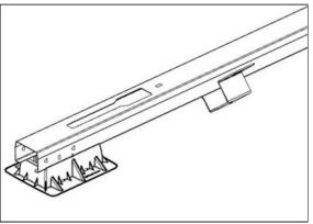
1. Place the clamp bracket with the lip upwards at the point where the lightning conductor will be connected.
