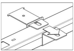
2. Slide the clamp plate into the clamp bracket.
