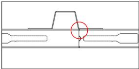
1. Place the bridging bracket over the connection. Ensure that the setting aligns with the transition between both beams. The screws will then leave the connection between both beams clear.
