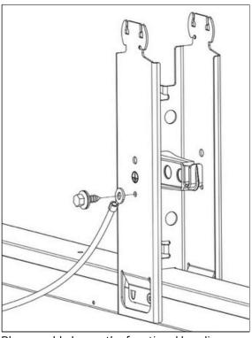
Place a cable lug on the functional bonding conductor.
