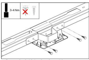
2. Screw the bridging bracket with the drilling mounting screws (IO1046).
