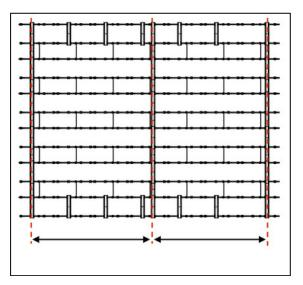
**NOTE!** Install additional rows of ballast plates for large fields to comply with the maximum separation distance, in accordance with Lightning Protection Class 1 (5x5m), 2 (10x10m), 3 (15x15m), 4 (20x20).
