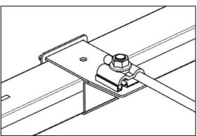
4. Tighten the nut to clamp the assembly onto the base unit (20 Nm).
