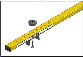
3. Use the size tool parallel to the ballast plate to keep the profiles at the right distance.
