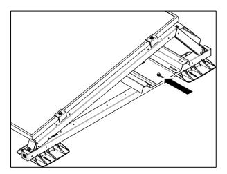
1. When mounting Sunbeam Nova, place the ballast plates more inwards or grind them down so that they are flush with the base unit.
