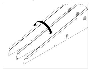
3. Fold over the top edge of the side plate. You can use the side plate for both the left and right sides of the mounting system.
