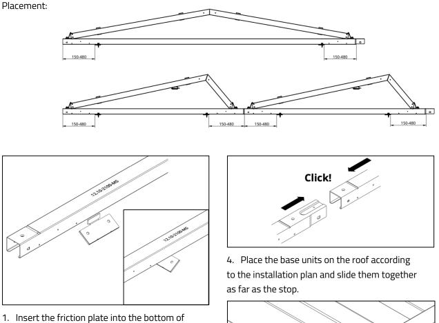
1. Insert the friction plate into the bottom of the base unit.
